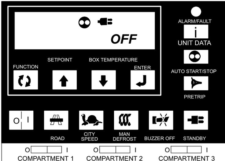
The microprocessor will power up and go through a self test. It will then show “OFF” in the display.
