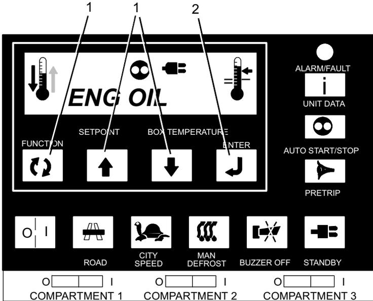
1. Press the FUNCTION key and then the UP or DOWN arrow key until ALARM RST is displayed.
