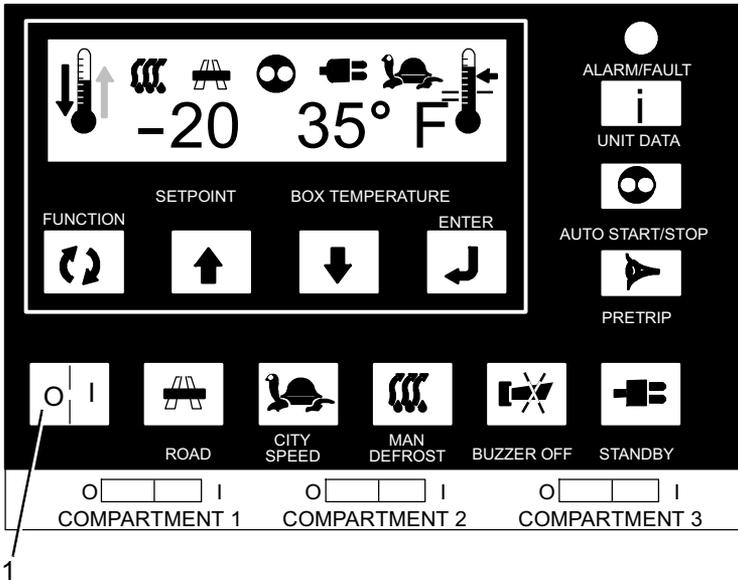
1. To stop the unit, place the I/O switch in the “O” position or place the unit RUN/STOP switch in the “STOP” position.
