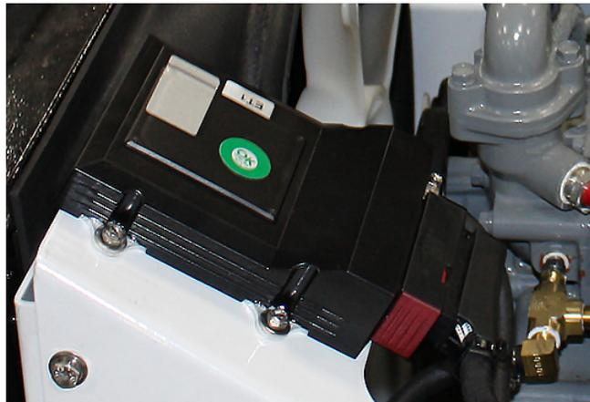
The ECM will signal to the service light, [Figure 3.8](#), as part of alarm notification. A unit with an illuminated service light indicates immediate service is needed, and will continue to operate for up to 250 hours in order to protect load and allow adequate time for delivery. After 250 hours, the unit will shut down until the EES is repaired.
